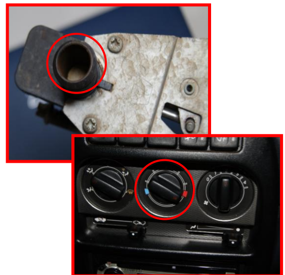
Ensure valve is opening and closing when heat dial is operated
