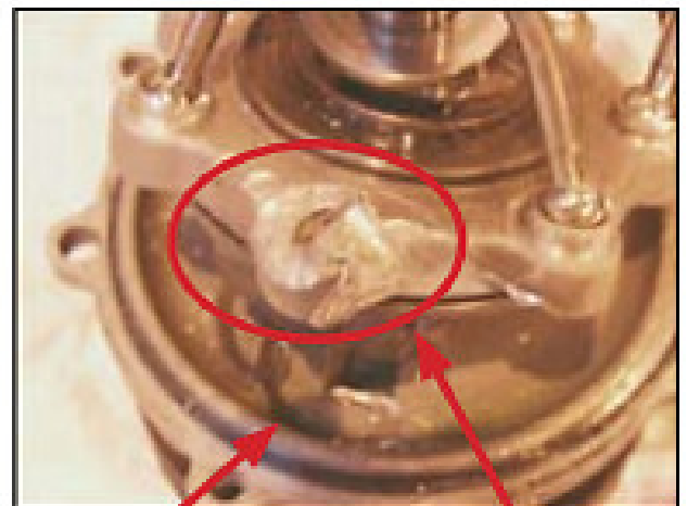
Damaged piston rings
