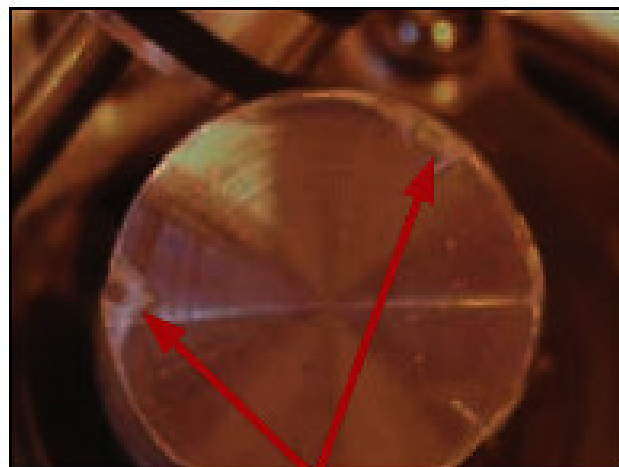
Damage to piston crown
